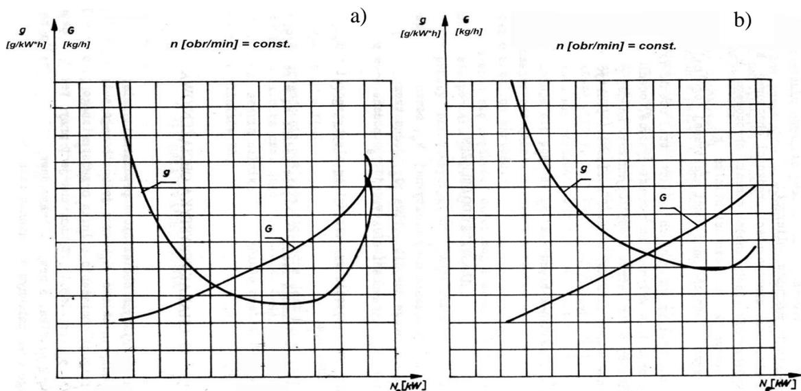
Fig 1. Load characteristic: a) compression ignition engine, b) spark ignition engine
